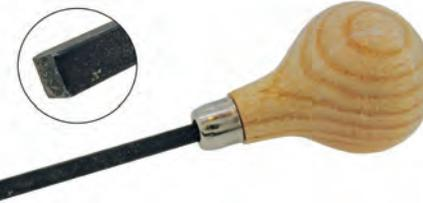
Super prong pusher tool used to push metal over the stone. It is made of soft steel to reduce the risk of damaging the stone.
