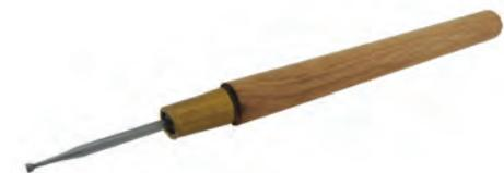
The Designer Wire Rounder has a small cup burr at its tip that rounds wire ends.
