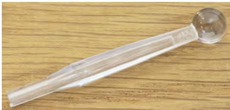
A simple instrument used to observe interference figures in gemstones such as quartz, the Conoscope Rod is used in conjunction with a polariscope to determine whether the stone is uniaxial or biaxial.
