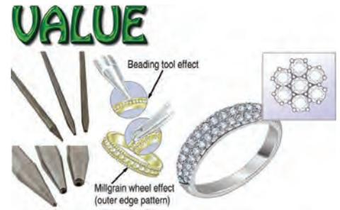
Bead Patterning: For producing a sphere / ball shape final finish to the end of the grain setting and also for creating decorative miniature ball patterns & wire end rounding.
