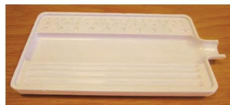
Sorting tray is used to sort stones, diamonds and pearls etc. It has various shapes of grooves and lines to aid efficient sorting.
