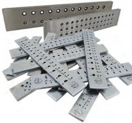
A draw plate is a multi-die plate made of hardened steel which wire is drawn through to thin it. Our Draw Plates are available in many different shapes and sizes including round, square, oval, half-round rectangular square and triangular for reducing and forming different shaped wire. The drawing holes on the plate are wider at the rear and taper slightly towards the front.
