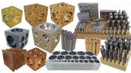
Our variety of dapping blocks, cubes, punches & sets makes forming and doming sheet metal into shapes adding dimensions and depth to designs simple. Made in various materials metal, brass, rubber and wood, we cater for all types of working material and practices.
