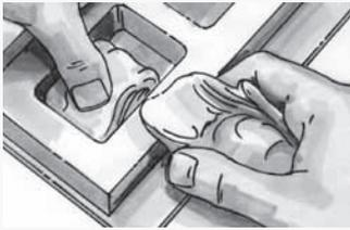
Castaldo Silicone Molding Rubber is soft and pliable, with a consistency like putty or molding clay.
