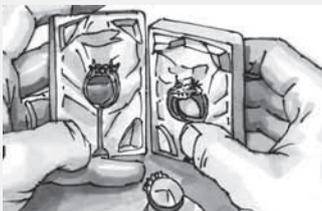
Finished molds can be simple or complex with cores, straight plugs or even spiral plugs. Castaldo Silicone Jewelry Rubber Molds are strong and tear resistant and can last for years and years.
