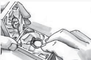
Parting lines are easily controlled and corrected by hand when used with the powder separation technique.
