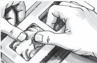
Curing Castaldo Silicone Jewelry Molding Rubber involves no mixing, limited working times or de-bubblizing. Simply put into your vulcanizer between 160°F - 190°F (71°C - 88°C) for 15 minutes per 1/4 inch (6mm)
